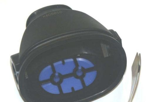
Be sure to closely inspect the second stage case around the lever support area for cracks. This is a high stress area and can be damaged if the regulator becomes snagged during entry or exit from the water.
