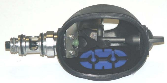
Lightly stretch the diaphragm between your fingers to inspect for holes.
