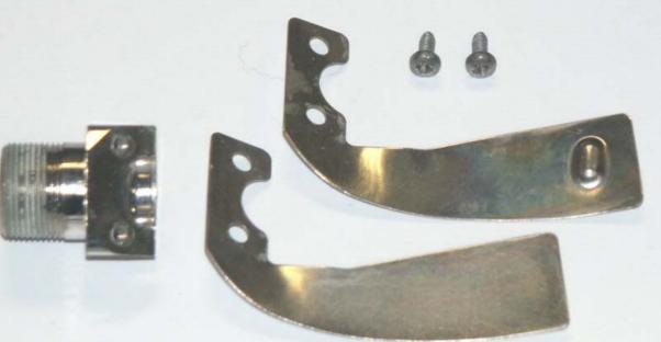
The moisture retention fins should last the life of the regulator and never need to be replaced. If they do become damaged, they can be with a phillips head screw driver. ONLY IF NEEDED USING THE OLD LP SEAT, REVERSE THE PROCEEDURE TO REASSEMBLE. REPLACE THE POPPET SCREW, P/N 73-5602-4, WITH A NEW ONE.
